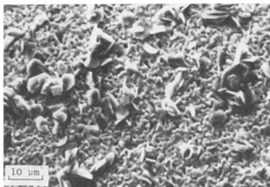
Figure 8 Surface of metallizing fired on alumina X first in wet hydrogen and then in dry hydrogen (SEM).
